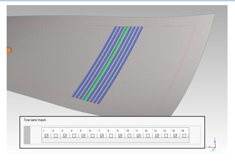
Added the ability to define which tows are active while laying tape in **Setup -> Head**.
